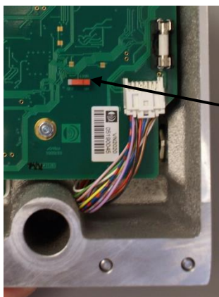
Figure 52: Switchable termination resistor
