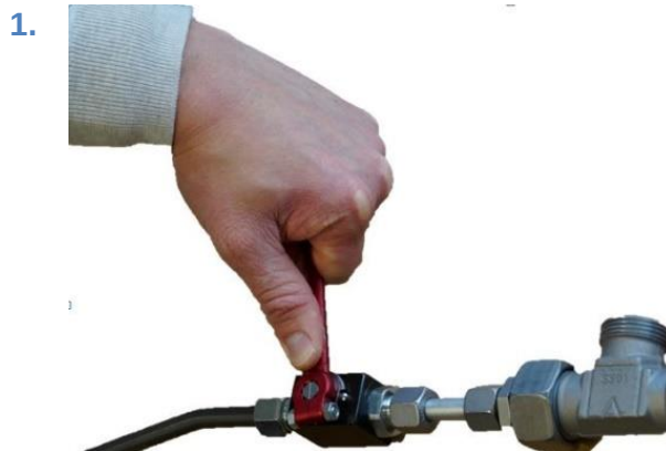
Figure 154: switch off compressed air
