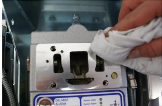
Figure 69: cleaning sealing surface
