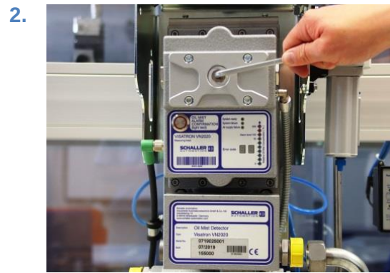
Figure 181: Inspection cover with mounted quick coupling cover
